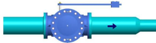
Swing Check Valve should be installed a minimum of 6 diameters downstream of a reducer/expander or bend to ensure flow at valve is fully developed and turbulence is minimised.
