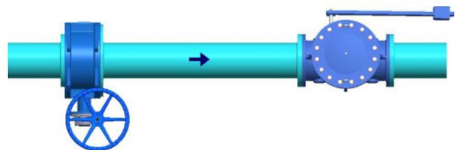
Swing Check valves can be installed close to an upstream or downstream non-throttling isolation valve (e.g. VOSA Full Port Wedge Gate Valves).
