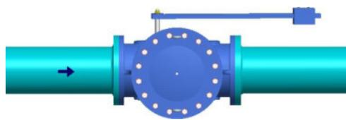
VOSA Swing Check Valve most suited for horizontal flow with disc directed towards the flow.
