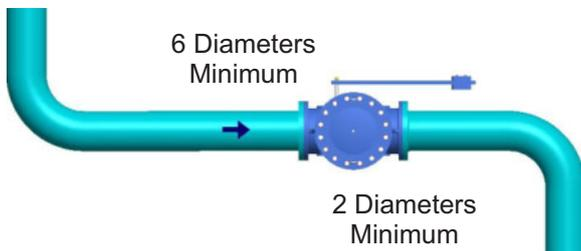
Swing Check Valve should be installed a minimum of 2 diameters upstream of a reducer or bend to avoid choked flow, which would cause the valve to only partially open
