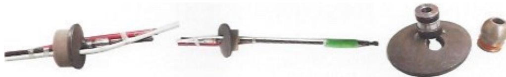
Left to right: 25T PLV Mechanical Anchor with dome plate, grout tubes & foam sponge; 25T Mechanical Anchor DTI Barrel with dome plate, grout tubes, foam sponge, anchor shell & cone; 25T PLV with dome plate, untensioned (snap ring attached); 38T PLV excluding dome plate, tensioned (no snap ring)
